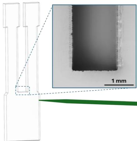
Figure 1. QTF design used for processing. The inset shows an optical microscope image of the facets at the support-prongs junction of the QTF.
