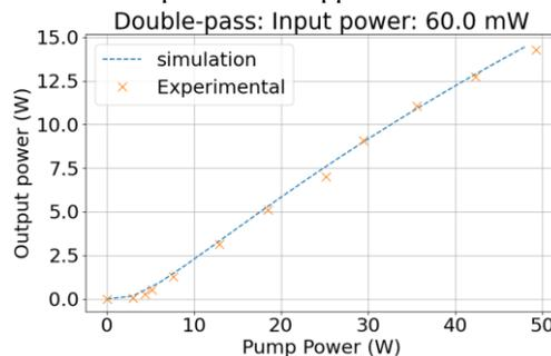
Figure 2: Measured (x) and simulated (dashed line) amplifier output power vs pump power, for a narrow band CW seed of 60 mW input power.
