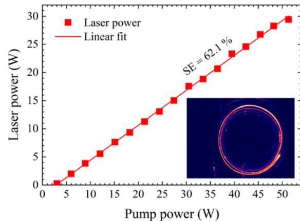
Figure 1. Performance of the segmented fiber laser and a thermal camera image.
