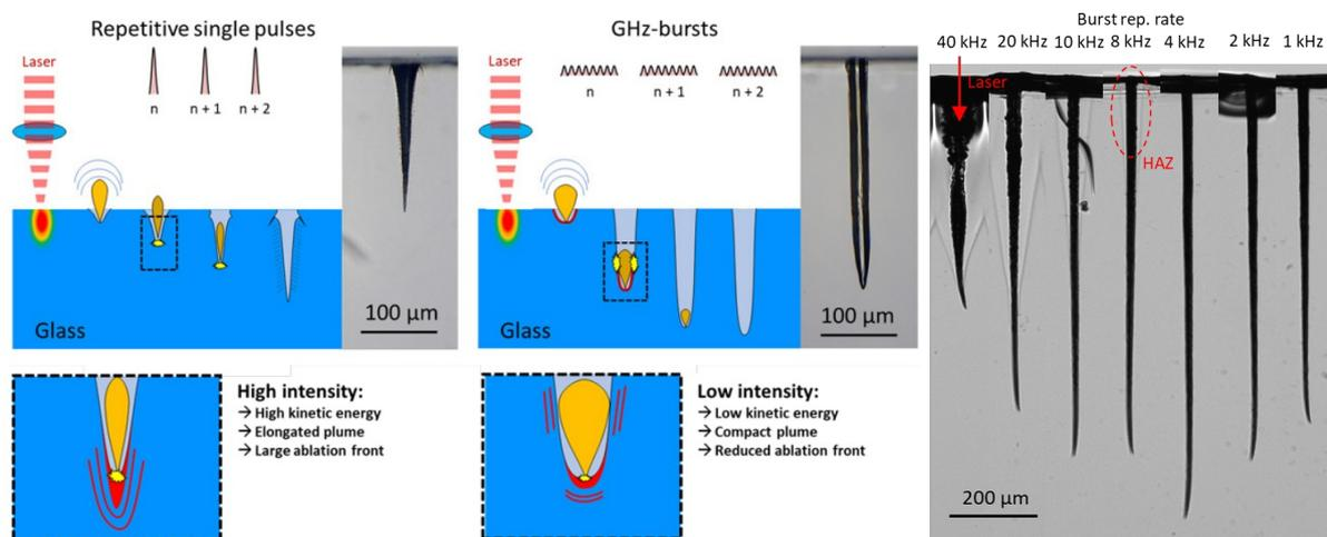
**Fig. 1** (left) Schematic representation of the drilling process in the repetitive single pulse regime and in the GHz-burst mode [3]. (right) Micro drilling of Eagle XG glass at 1.28 GHz, heat affected zone and crack appearance with increasing burst repetition rate.
