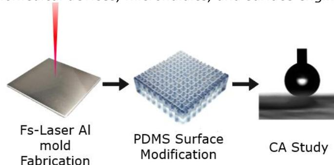
**Figure 1:** Graphical diagram of the process. (a) Femtosecond laser aluminium substrate texturing; (b) modified PDMS surface after the curing process [3]; (c) C.A. study and surface characterization.
