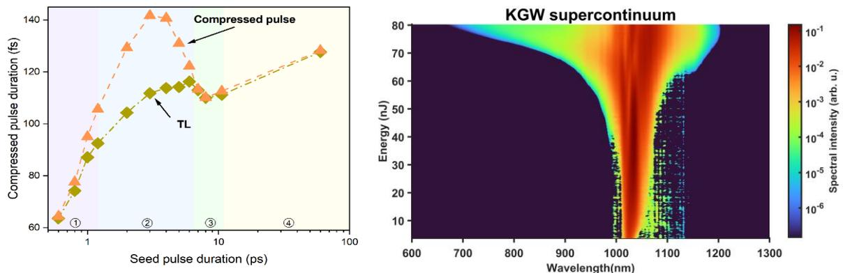
**Fig. 1** Left – compressed amplified pulse duration dependency on initial pre-chirp value. Right – supercontinuum spectrum generated from KGW crystal.
