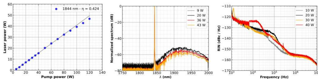
**Fig. 2** Laser output characterization: (a) power, (b) spectra, and (c) RIN.
