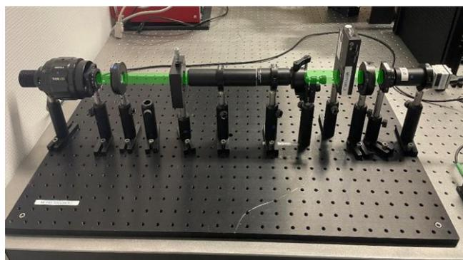
Fig. 1: Automated monochromatic circular polarimeter set-up
