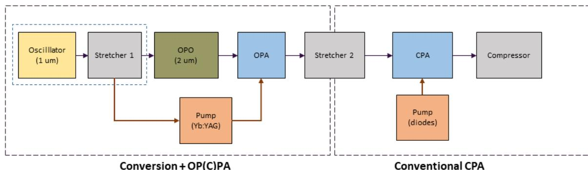
Figure 1: Proposed architecture for a high average power ultrashort pulse laser at  $2\mu\text{m}$  wavelength.
