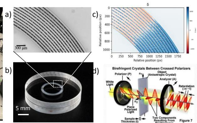
Fig. 2: (a) Micrograph of the sample to analyze with Patterson and Wang 6-step method. (b) Picture of the full sample, 3 mm-thick fused silica windows welded with ultrafast laser, the welding pattern is a donut. (c) Optical retardation (nm) of the bonded sample. (d) Scheme of birefringent crystal placed between two crossed polarizers [4].
