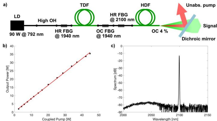
Fig. 1 a) Experimental setup. b) Measured output power and linear fit with 80 cm fiber. c) Output spectra at full power.
