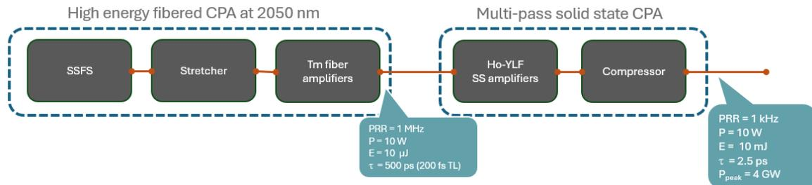
Figure 1: Hybrid CPA system design
