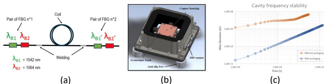
**Fig. 1** Sketch of the two wavelengths resonant FBGs cavity (a). Packaged cavity (b). Cavity stability improvement using passive packaging (c).
