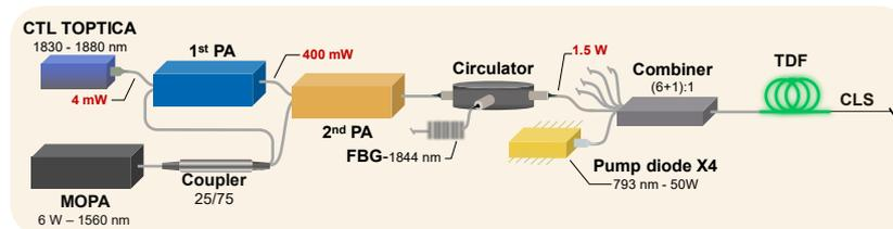
**Fig. 1** Schematic of the three all-fiber amplification stages. SF; MOPA – Master Oscillator Power Amplifier; FBG – Fiber Bragg Grating; TDF – Thulium-Doped Fiber; CLS – Cladding Light Stripper.
