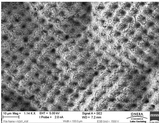
**Figure 1 – SEM image of Laser Texturing by Direct Laser Interference Patterning (DLIP) on suspension plasma-sprayed ("SPS") YSZ.**
